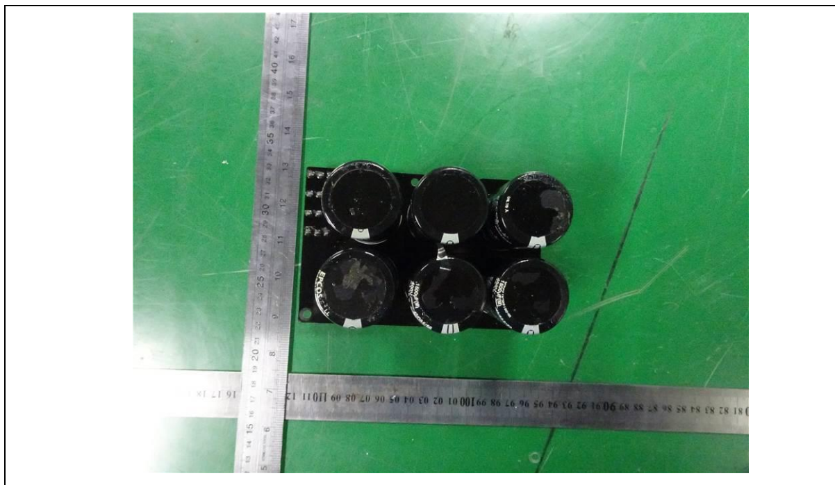
Details of: Components side view of Bus cap. board (Model GD20-022G-4)
