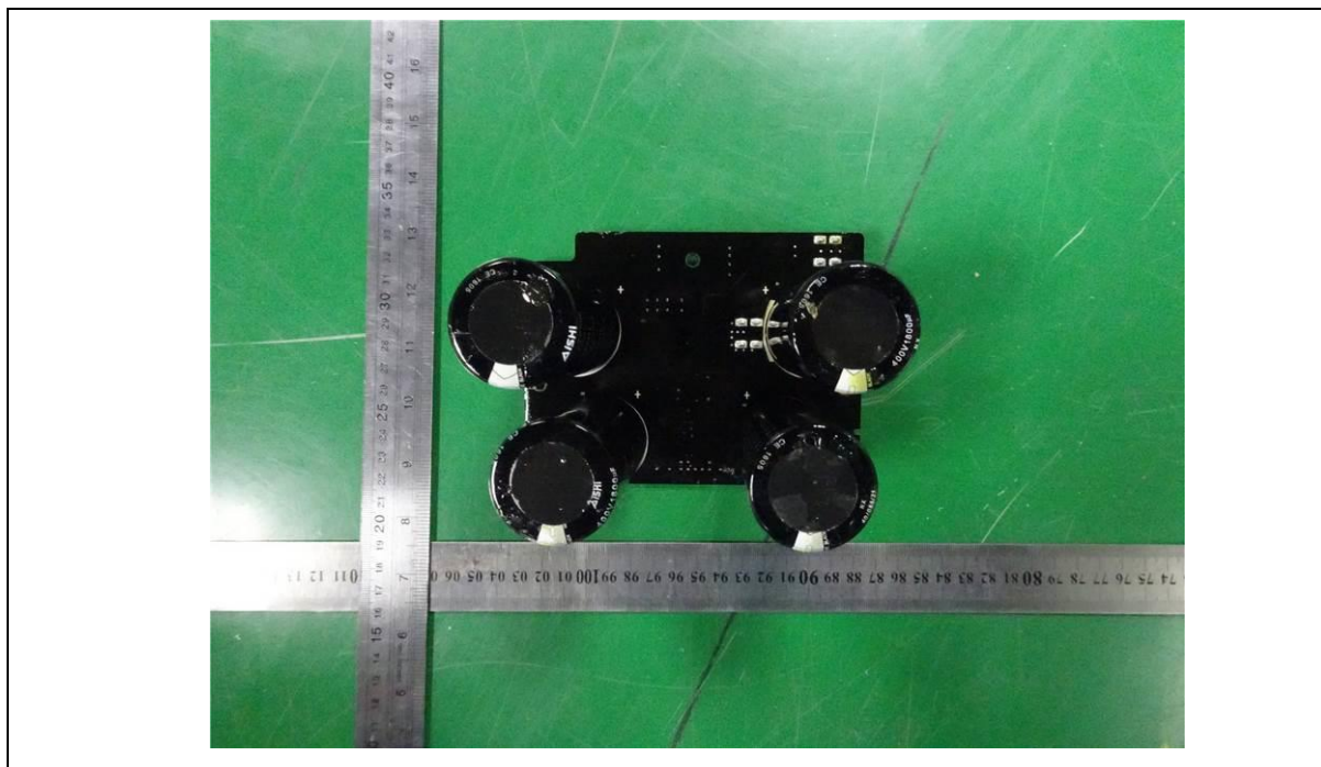
Details of: Components side view of Bus cap. board (Model GD20-015G-4)
